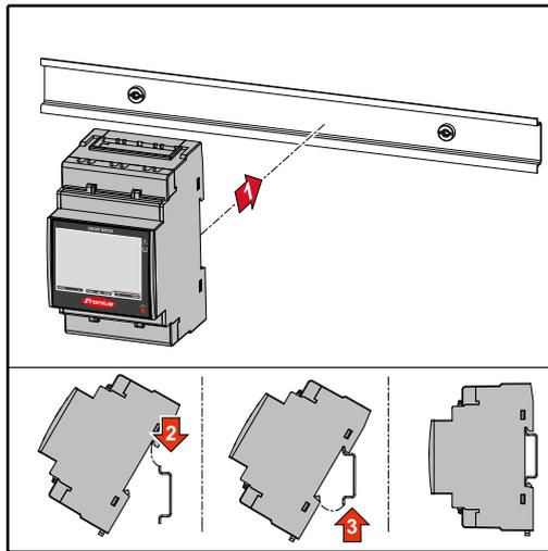
The Fronius Smart Meter TS can be mounted on a 35 mm DIN rail. The housing comprises 3 modules according to DIN 43880.
