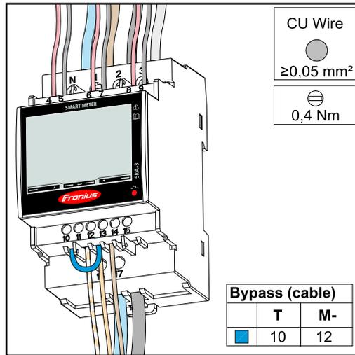
The terminating resistor is integrated in the Fronius Smart Meter TS and is manufactured with a bridge between the M and T connections (T = termination).
