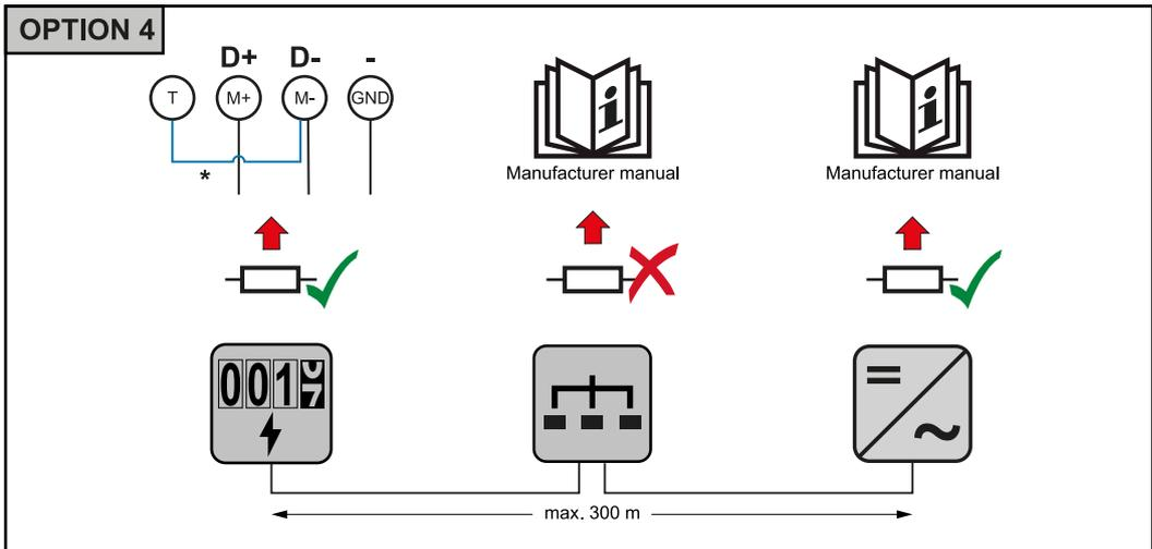
\* The terminating resistor is integrated in the Fronius Smart Meter TS and is manufactured with a bridge between the **M** and **T** connections (T = termination).
