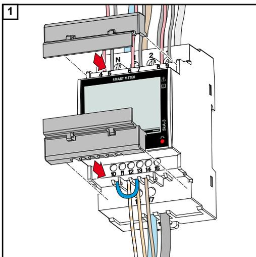
Insert the connection covers into the guides and press firmly.
