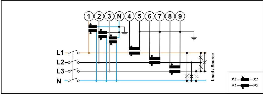
3 phases, 4 conductors (VT/CT connection)
