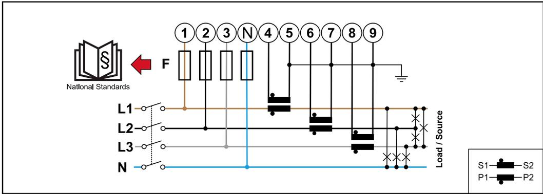
3 phases, 4 conductors (CT connection)
