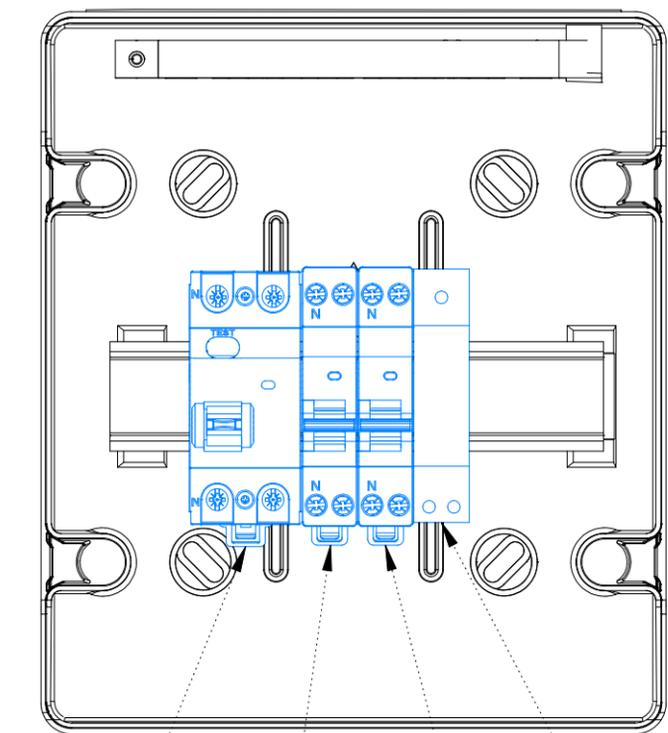
INTER DIFFERENTIEL    PROTECTION ONDULEUR    PROTECTION PARAFoudre    PARAFoudre
